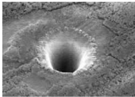
Figure 13: SEM micrograph hole drilled in 250 micro meter thick Silicon Nitride with 3 rd harmonic Nd: YAG laser
