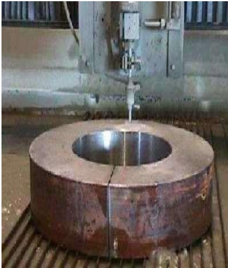
Abrasive water jet cutting
