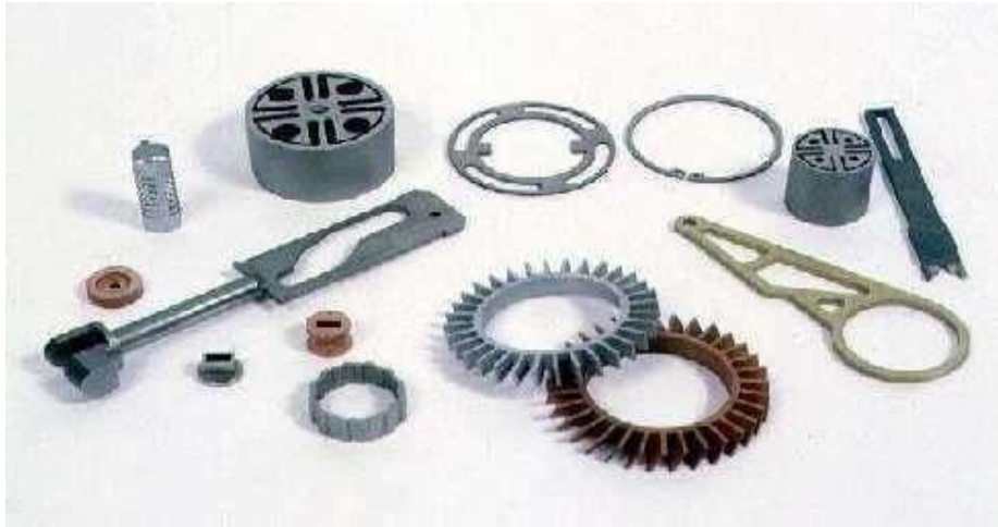
Figure 3: Difficult internal parts made by EDM process working
