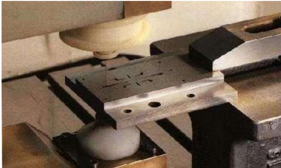
Figure 4: Wire erosion of an extrusion die
