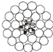
Fig 1.1 Cross-section of typical ACSR conductor.
