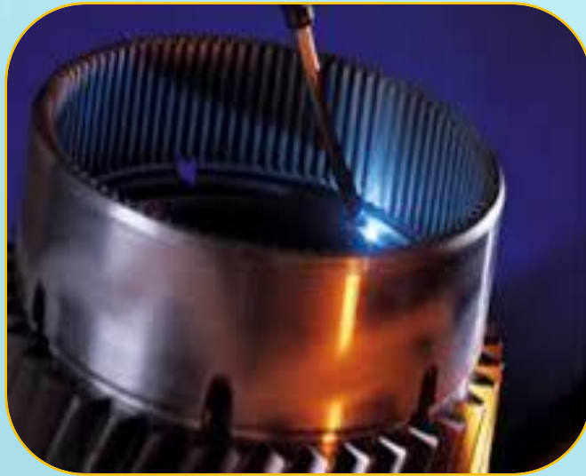
Laser surface treatment to change the micro structure of metals through controlled heating and cooling.
