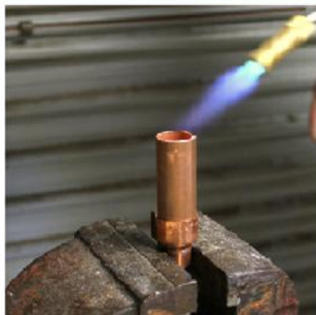
Fig.9.3 Hard soldering of copper with brass
