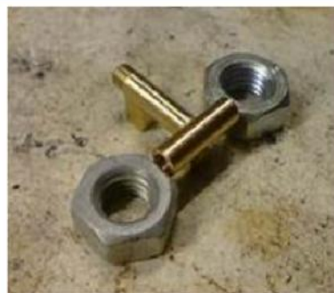
Fig.9.4 Hard soldering of stainless steel with brass
