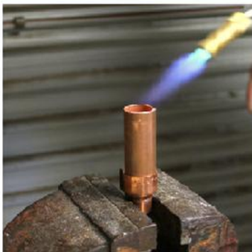
Fig.9.3 Hard soldering of copper with brass
