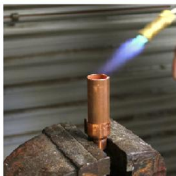
Fig.9.3 Hard soldering of copper with brass
