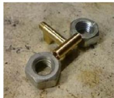
Fig.9.4 Hard soldering of stainless steel with brass
