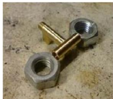
Fig.9.4 Hard soldering of stainless steel with brass
