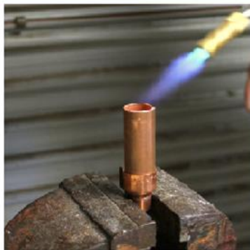
Fig.9.3 Hard soldering of copper with brass
