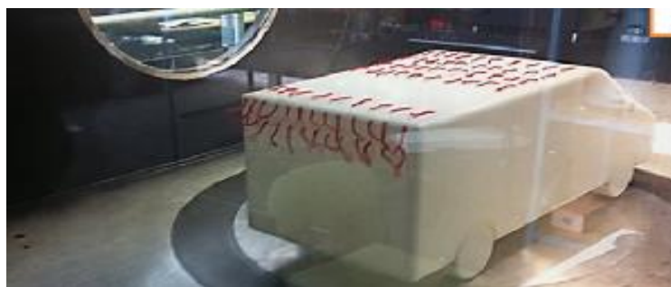
Fig. 8: Tuft flow visualization over the model car
