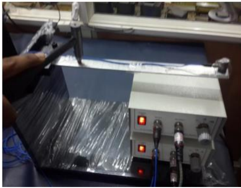
Fig 12.2: Showing impact loading with hammer
