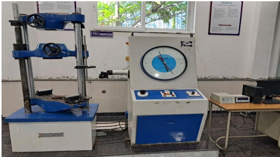
Fig. 8.1: UTM Machine for finding young's modulus
