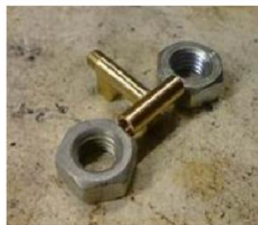
Fig.9.4 Hard soldering of stainless steel with brass
