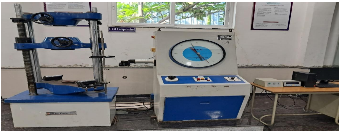
Fig. 7.2: UTM machine for finding shear stress
