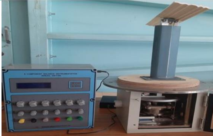
Fig.13: Six component balance with display and strain gauges
